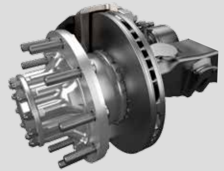
Ventilated discs reinforce safety
